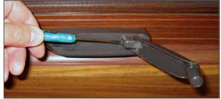
Use a small screwdriver to remove the handle.
