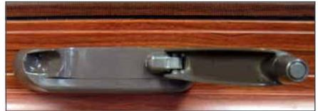
Crank in unfolded position.
